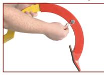
After checking the roof pitch, match the pitch to the etched number and lock it in place.
